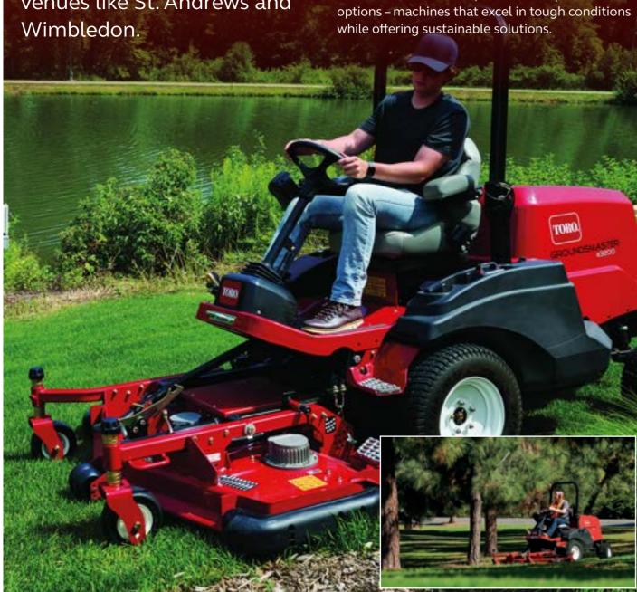
Flail mowers, like the Toro LT-F3000, handle dense vegetation with Tempest™ flail blades, ensuring a clean cut and healthier regrowth. Cylinder mowers, such as the LT3340, deliver precise, scissor-like cuts for fine turf. Rotary mowers, including the Groundsmaster
