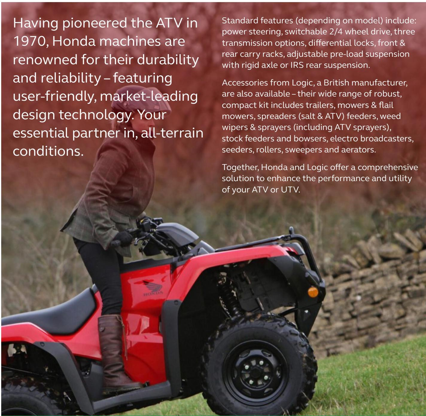
Standard features (depending on model) include: power steering, switchable 2/4 wheel drive, three transmission options, differential locks, front & rear carry racks, adjustable pre-load suspension with rigid axle or IRS rear suspension.
